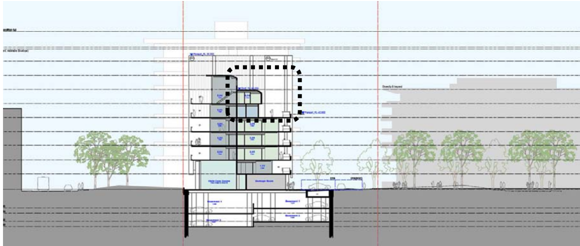
Figure 34: Section through the building showing where the deletion of bulk occurs to maintain solar access to Block B.
